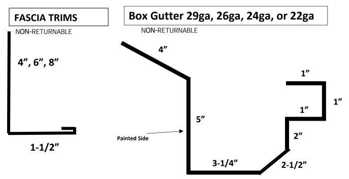
Does not include Ends, you will need to fabricate your own ends using a hand bender.
